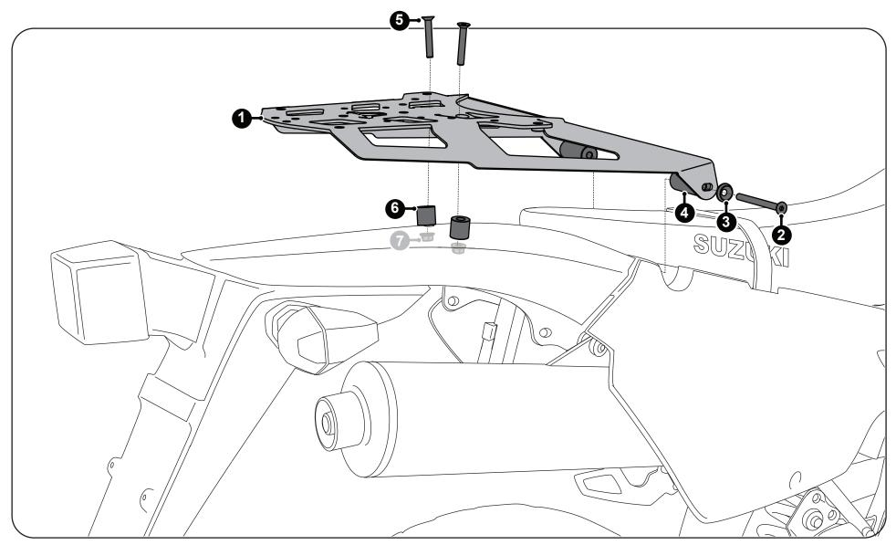
**Step One:** Remove the OEM tail bag and rear seat bolts. Loosley mount the front of the Steel Rack to the rear seat mounting points on your bike.
